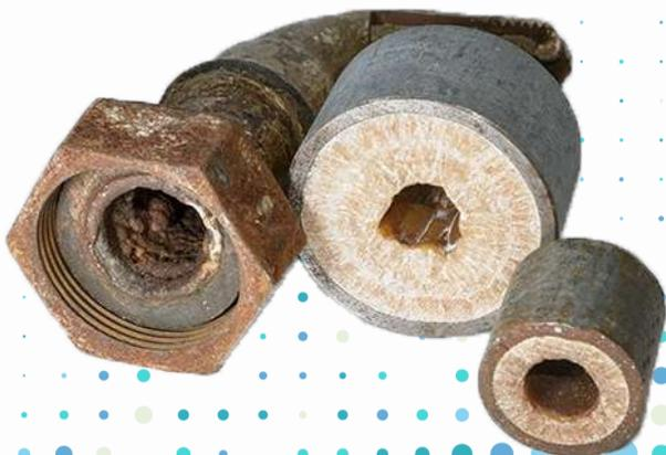
A single millimeter (**1mm**) of limescale in pipes carrying hot water can increase energy consumption by **10-15%**
